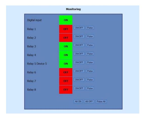
The "Monitoring" page provides information about the state of the relays and digital input.
